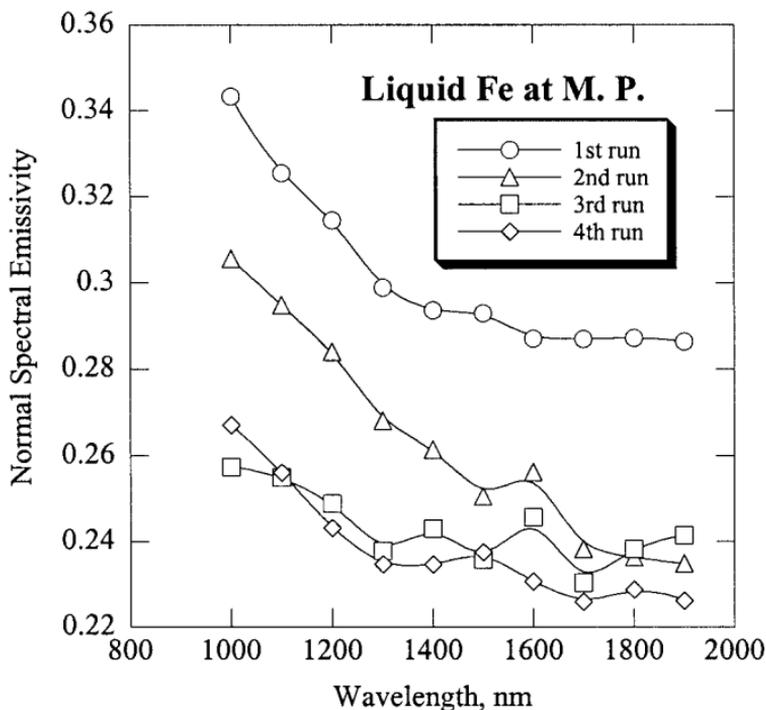
Fig. 3. Change in emissivity with number of measurement run for liquid iron heated in a flow of hydrogen.
